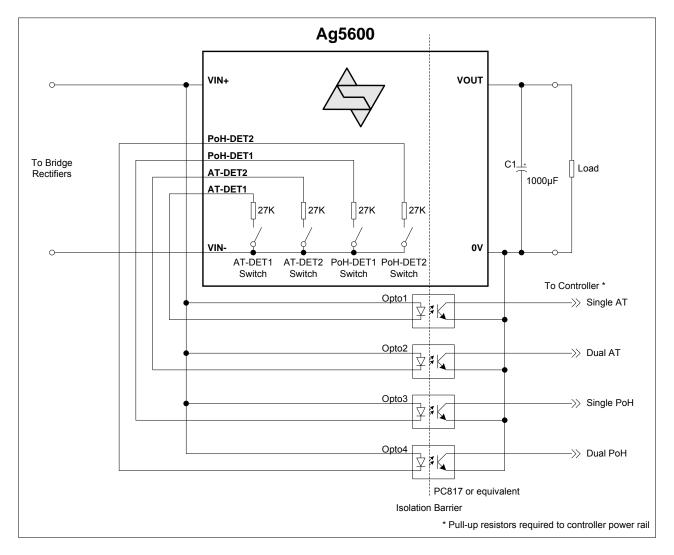
Figure 4: 2 - Event Physical Layer Detect Configuration
