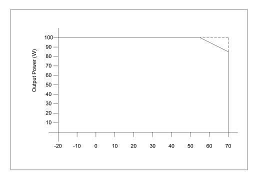
Figure 9: Ag5600 Operating Profile with Heatsink
