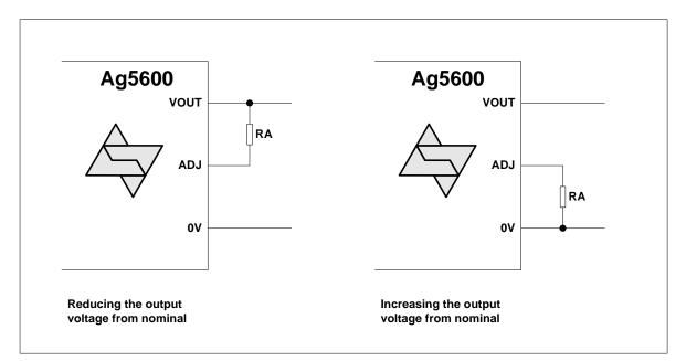
Figure 5: Output Adjustment
