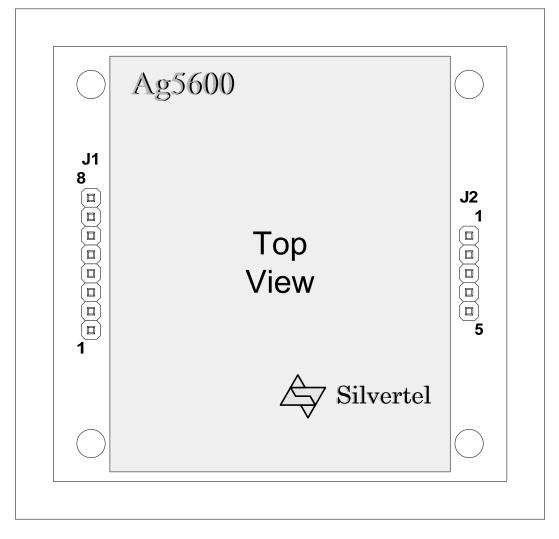
Figure 2: Ag5600 DIL Package Format (Top View)
