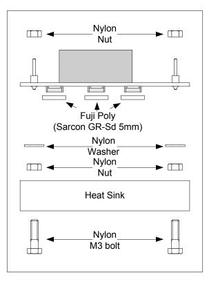
Figure 8: Suggested Heat Sink Assembly
